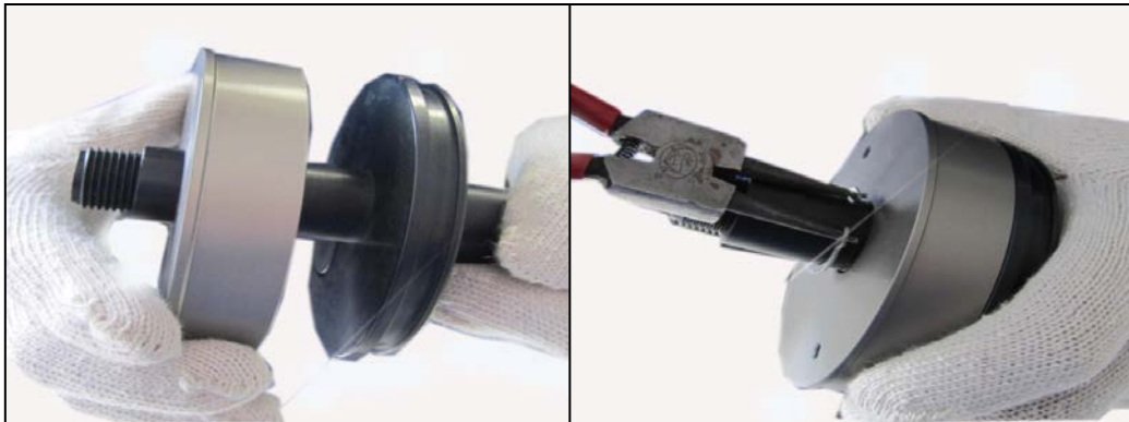
Figure 2.14 Bearing plate installation
