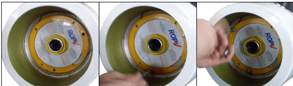
Figure 2.23 Install the retaining
