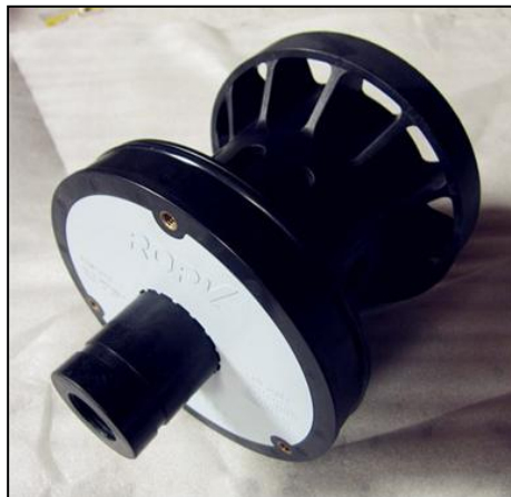
Figure2.13 Install the thrust ring
