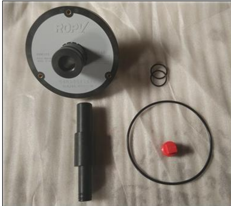
Figure 2.7 Head breakdown figure 1 (sealing plate)
