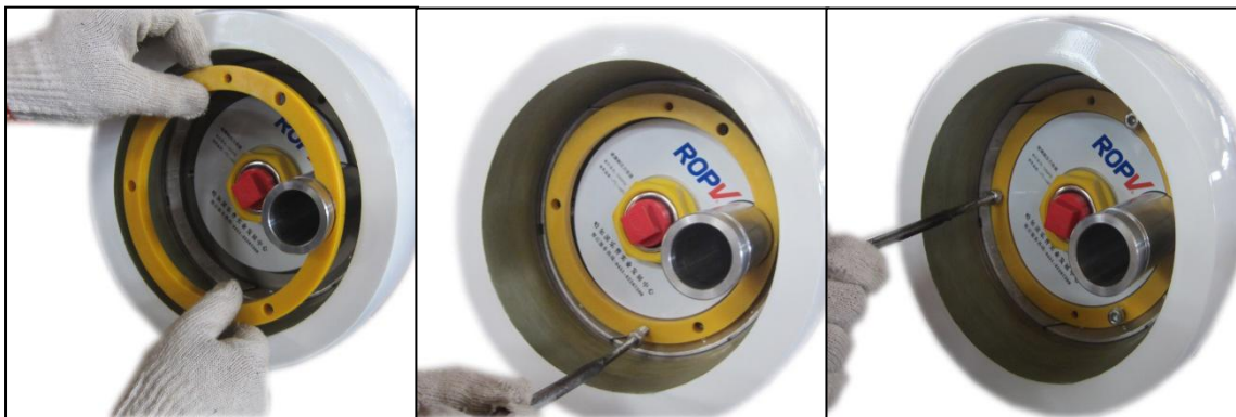
Figure 2.23 Install the retaining ring
