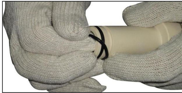
Figure 2.15 Adaptor seals installation
