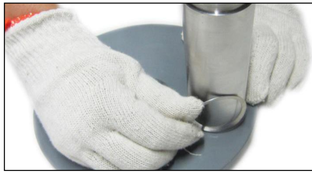
Figure 2.16 Installing feed/concentrate port
