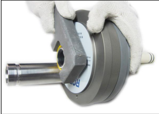
Figure 2.7 Remove the locknut
