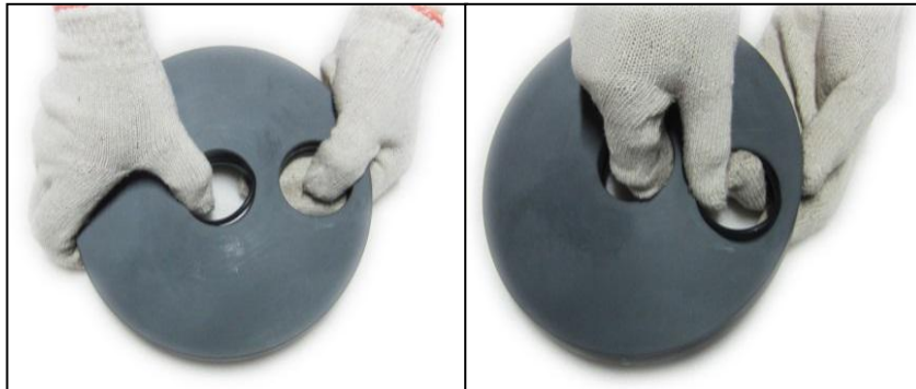
Figure 2.14 Install the sealing plate seals
