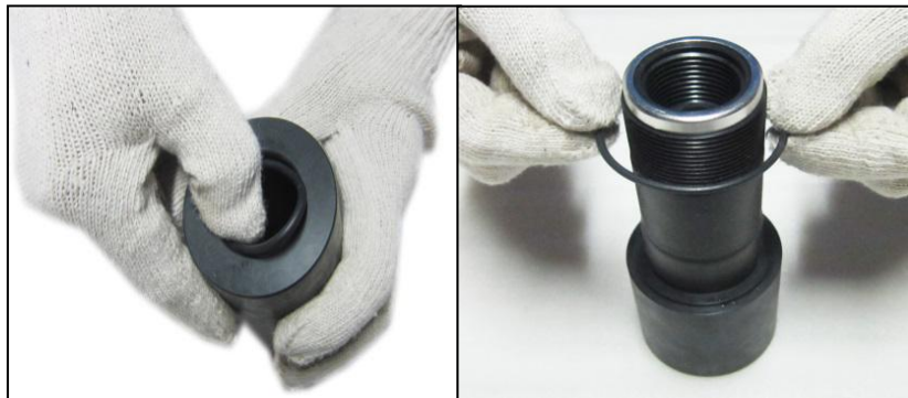
Figure 2.13 Install the permeate port seals
